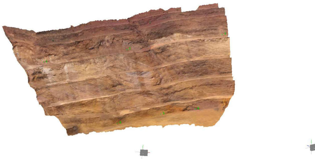
Figure 2 Surface model generated by 3DM Analyst. The six control points are in green.
