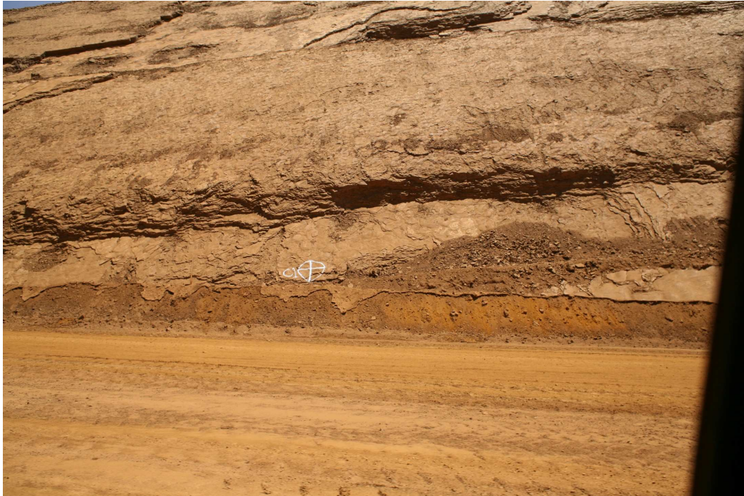
Figure 5 Image captured out the open window of a moving vehicle. Note the control point painted on the wall, and the vehicle's window frame on the right.
